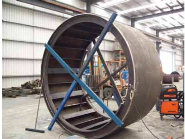
11000kg Thrust Ring for Tunnel Jacking
